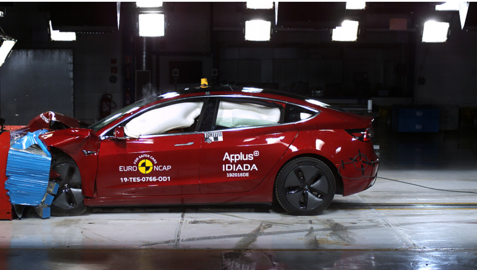
Tesla Model 3 Frontal offset impact test June 2019
