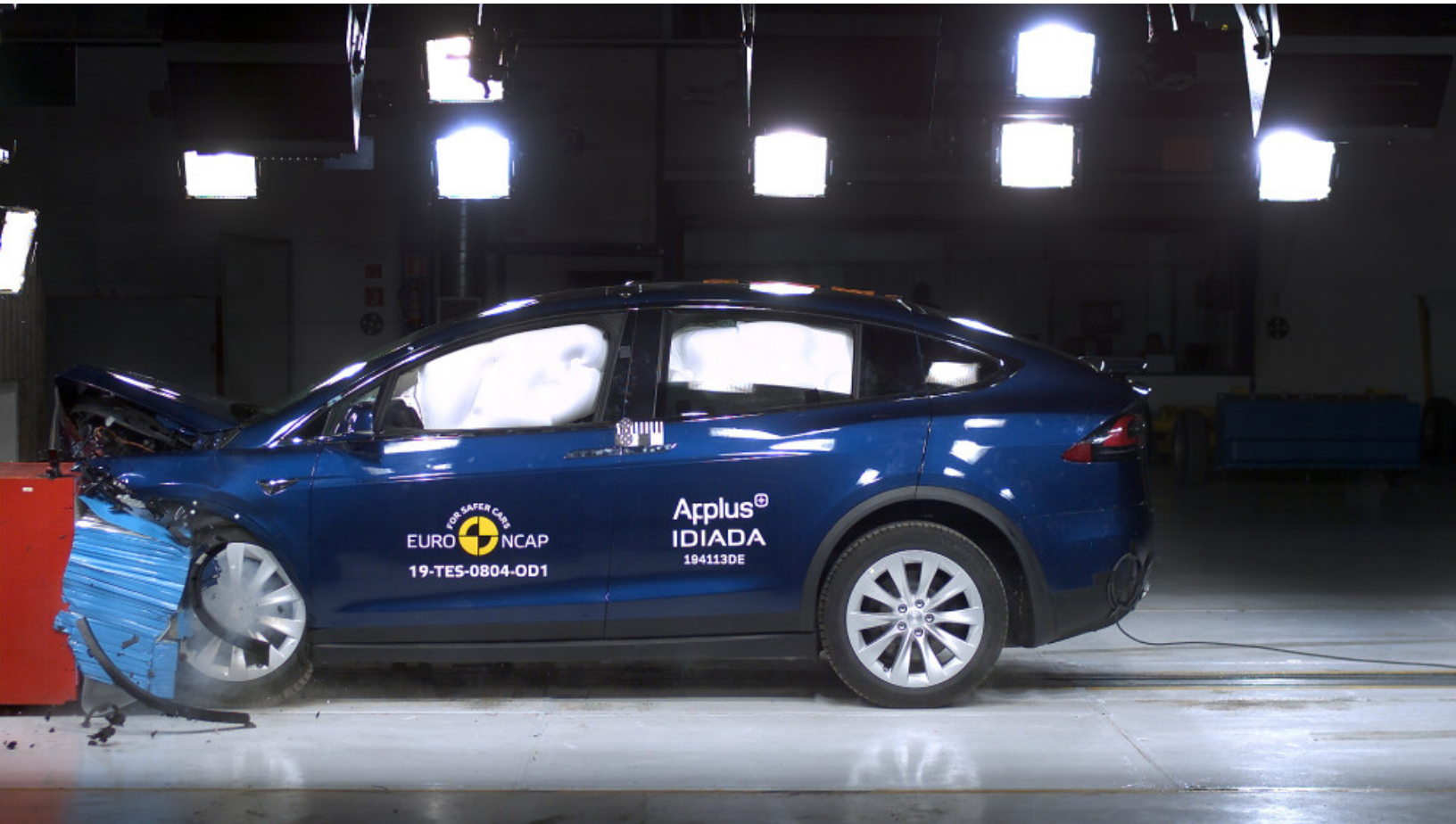
The Tesla Model X in Euro NCAP's offset deformable barrier test
