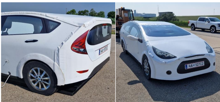
Figure 3: Front and rear views of the 4activeC2 car target.
