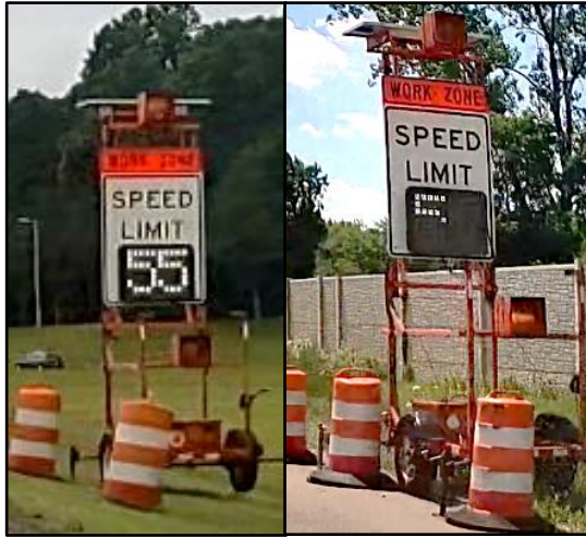
Figure 7: Flashing LEDs are used on some temporary speed limit signs. The difficulties caused by LED refresh rate can be seen in the right image.
