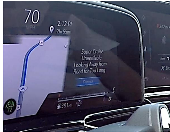
Figure 15: Visual information in the Cadillac Escalade when a distracted driver is detected.
