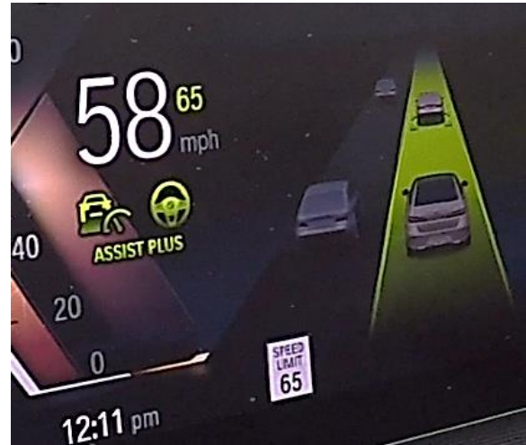
Figure 8: BMW i7 dashboard display showing the incorrect speed limit after passing a temporary LED sign.
