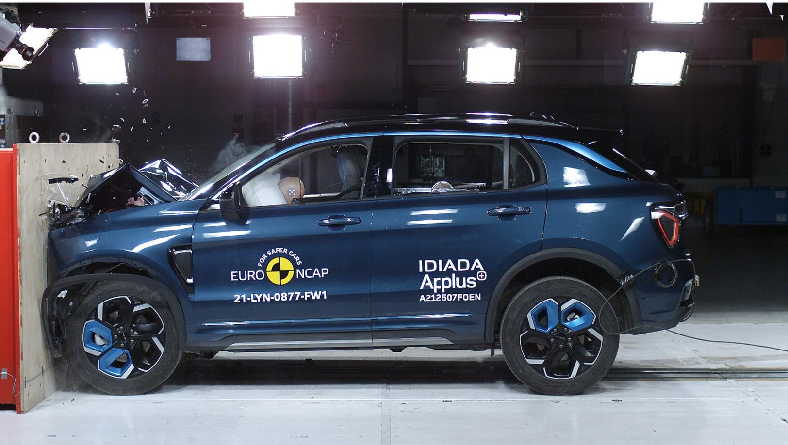
Lynk & Co 01 undergoes Euro NCAP's Full Width Barrier impact test
