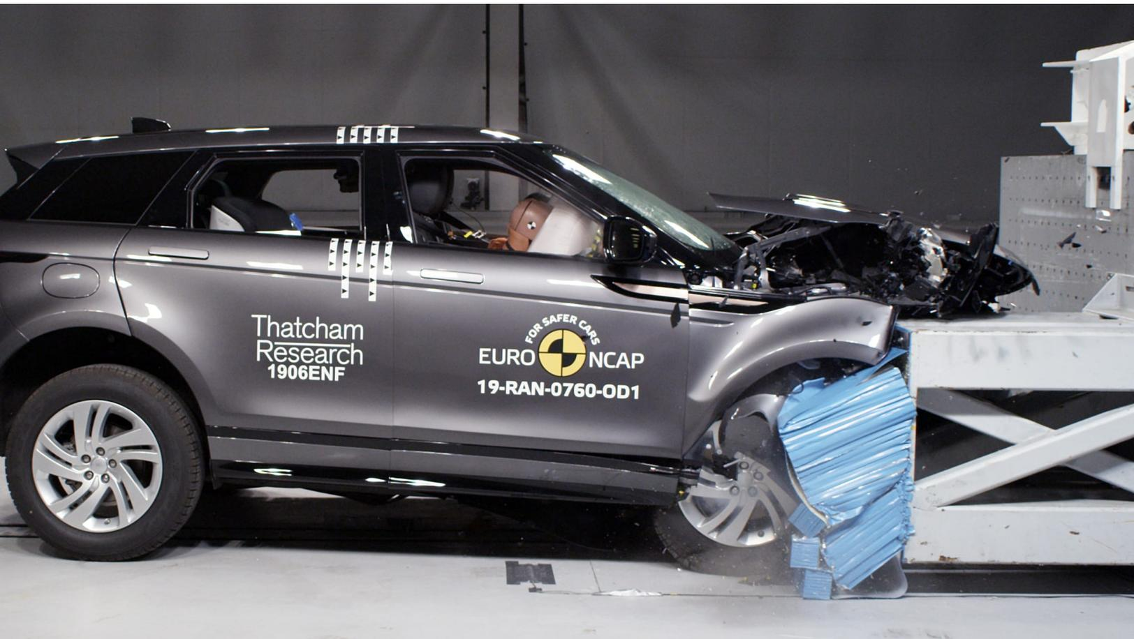
Range Rover Evoque Frontal offset impact test, April 2019
