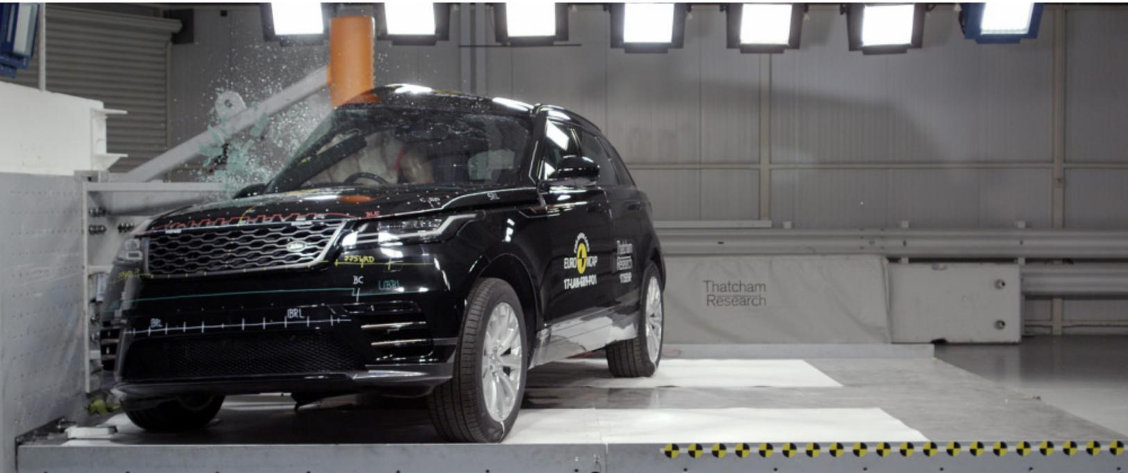
Euro NCAP's Side Pole impact test is a very severe test of a car's ability to protect the driver's head
