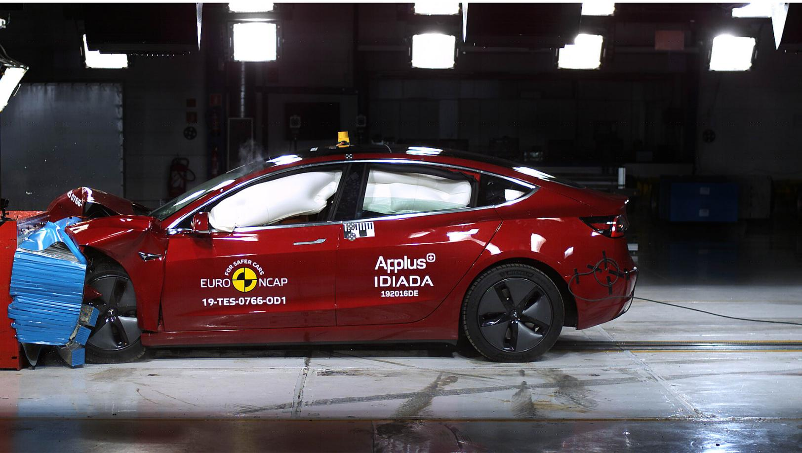
Tesla Model 3 Frontal offset impact test June 2019
