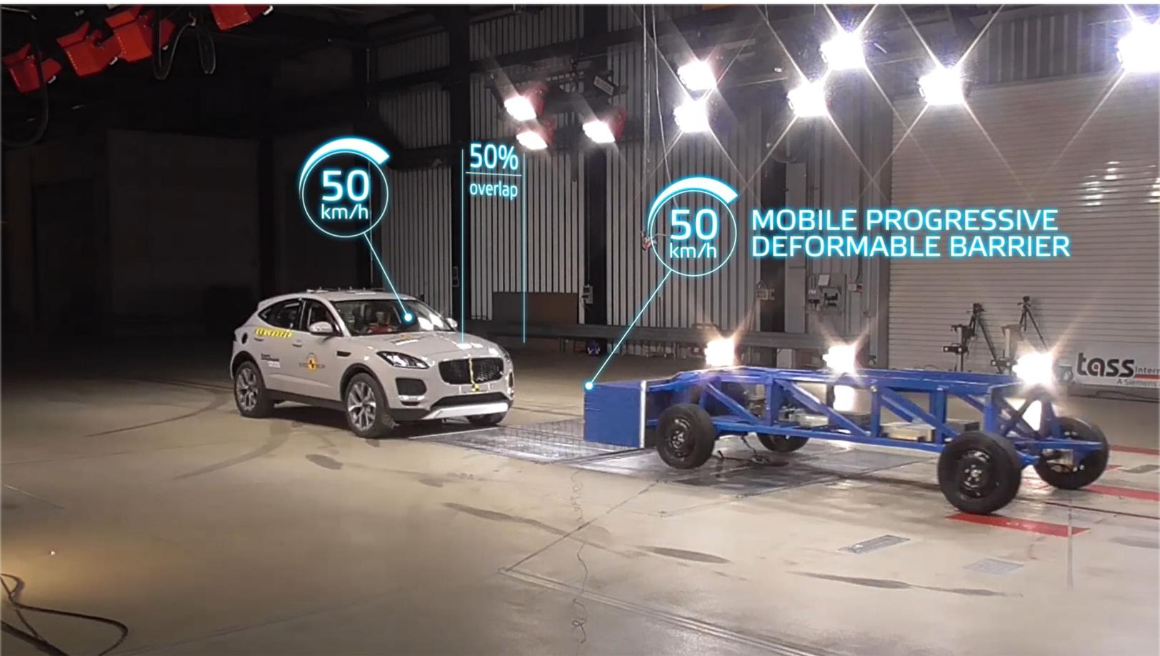
The new Mobile Progressive Deformable Barrier test
